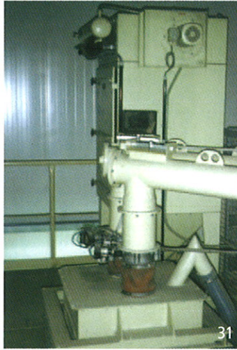
Pict.27: Double-flap free flowing gate for aggregate weighing scale. Pict.28: Feeding of 2 mixers by means of a two-way distribution gate underneath the aggregate weighing scale. Pict.29: Sizes and positioning of cement silos in all variations. Pict.30, 31: Optimal positioning of components on the weighing scale platform for optimal access. Pict.32: Feeding of 2 mixers by means of a two-way distribution gate underneath the cement scale Pict.33: Water weighing scale. Pict.34: Additive dosing scales in all variations.
